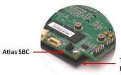
Thermally conductive heat spreader
