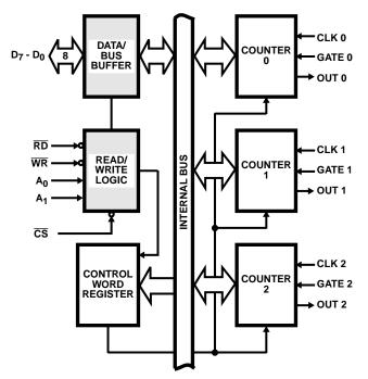
FIGURE 1. DATA BUS BUFFER AND READ/WRITE LOGIC FUNCTIONS
