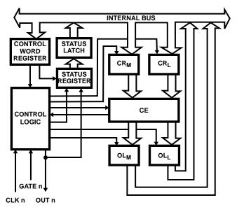
FIGURE 3. COUNTER INTERNAL BLOCK DIAGRAM
