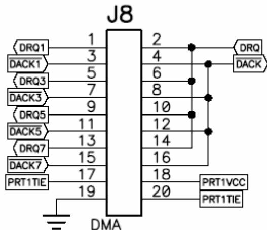
The signals DRQ and DACK# connect to the FPGA. Jumpers determine which PC/104 bus DMA channel is connected to the FPGA.
