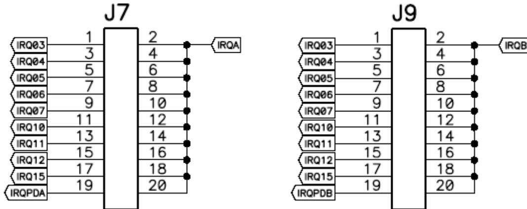
The IRQA and IRQB signals connect to the FPGA and can be routed through jumpers to the IRQx signals on the PC/104 bus.
