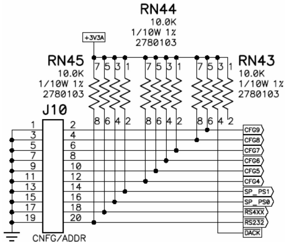
In the drawing above, SP\_PS1 = CFG3, SP\_PS0 = CFG2, RS4XX# = CFG1 and RS232# = CFG0.
