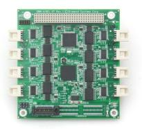
with programmable 120-ohm line termination. Each port is independently isolated with an isolated power + signal chip, plus additional isolators for control signals. The board features intelligent power management that limits inrush current on power-up and also enables power-down of unused serial ports for power savings.
