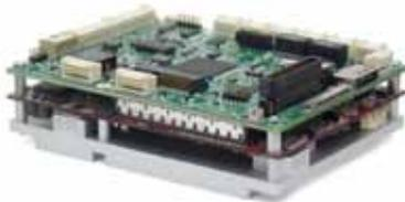
Vega offers EMX stackable I/O expansion. Its on-board PCIe MiniCard expansion socket facilitates the addition of an off-the-shelf mini PCIe add-on module, helping you satisfy your application's precise requirements.
