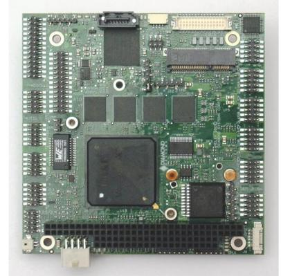
Helix supports stackable I/O expansion with PC/104 (ISA) I/O modules and also provides a PCIe MiniCard socket for additional I/O expansion. PCIe MiniCard I/O modules featuring WiFi, Ethernet, analog I/O, digital I/O, and CAN are available from Diamond Systems and other vendors, enabling compact expandability without increasing the total height of the system.
