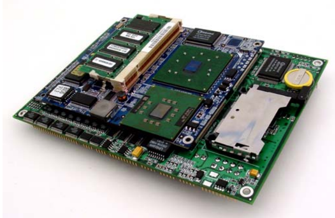
FIGURE 3. Neptune single board computer with an ETX CPU installed.
