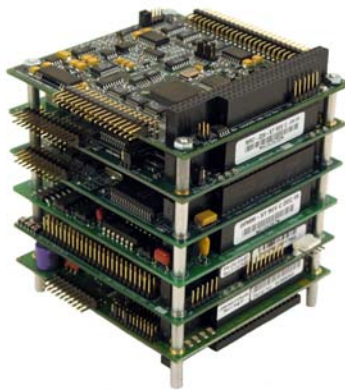
FIGURE 1: Older designs consisted of cumbersome stacks of CPU and I/O cards.
