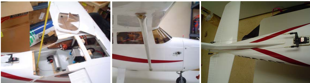
Figure 3. Airframe Modifications. Access Hatch (Left), Wing Struts (Center), Pull-Pull Rudder System (Right)
